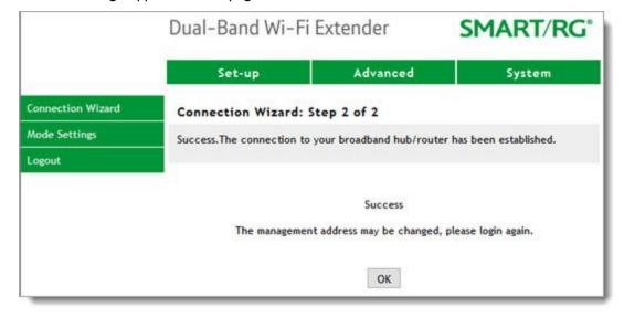
You are connected to the selected network. The WE65ac automatically detects and broadcasts the new SSID. A message about the management address appears. Click **OK**.
