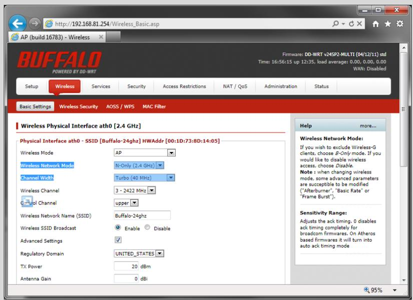
Under Wireless->Basic Settings, change *Wireless Network Mode* to “N-Mixed” or “N-Only” and change *Channel Width* to “Turbo (40 MHz)”.
