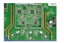
Non-adjustable internal PCB antennas Very small ~1-1.5 dbi gain
