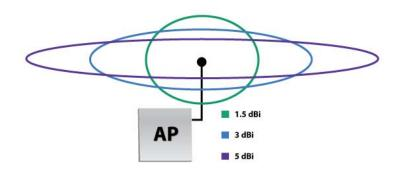
Vertical higher gain antennas have increased x-axis coverage at the cost of y-axis coverage
