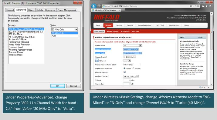
40 MHz operation in the 5 GHz spectrum is rarely an issue and is most often enabled by default on all products that are dual band.
